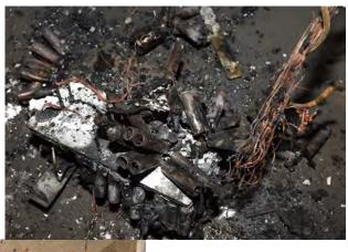
The fire at Bronx Box 77-2867 was determined to have been caused by an electric scooter's lithium-ion battery. (Photo by FDNY Bureau of Fire Investigation)
