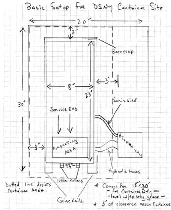
Figure 4: Diagram of space requirements for deployment of a compactor
