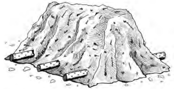
Passively aerated windrow
