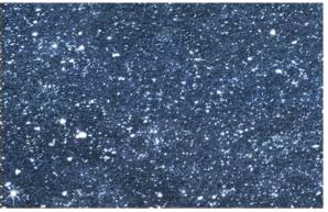
C.I.P Concrete, Type 4 Scofield Denim Blue Integral Color w/ Seeded Silica Carbide Aggregate Medium Smooth Finish
