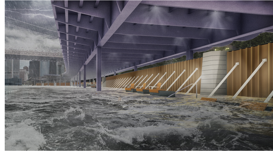
Flip-up gates activated during storm
