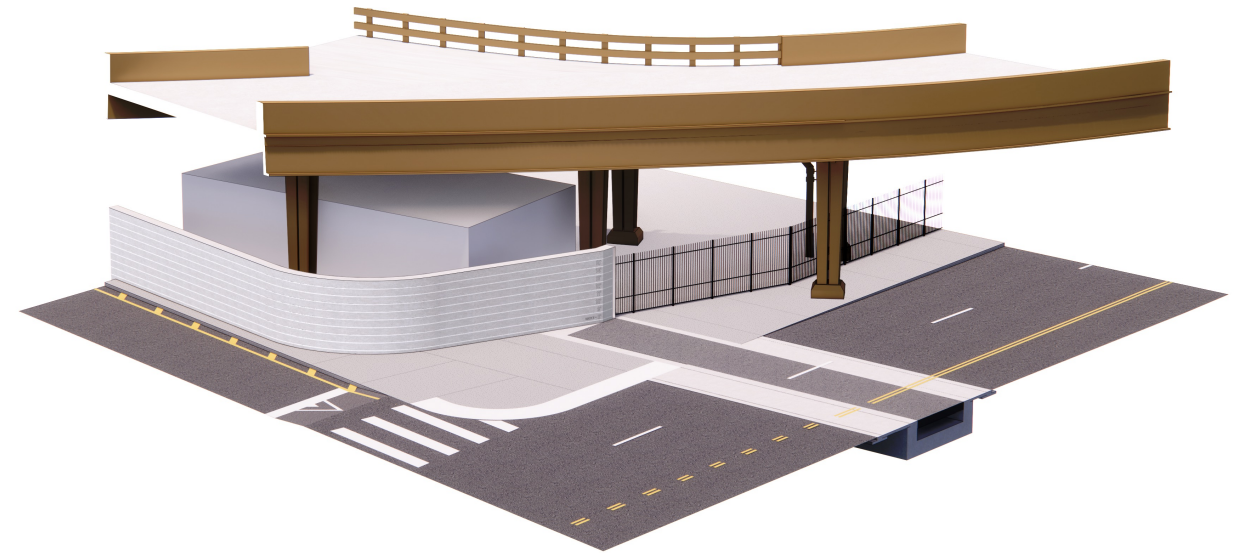
Rendering of floodwall tie-in and flip-up gate at South Street under Brooklyn Bridge From 2021 PDC Presentation :
