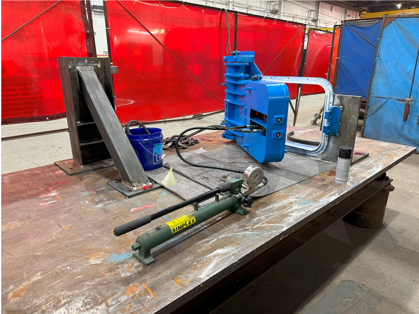
1/4 scale model interceptor gate, ready for NYC DEP testing – 2024
