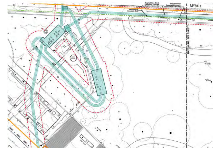
Detail of Water Mains and Vault Under Plaza
