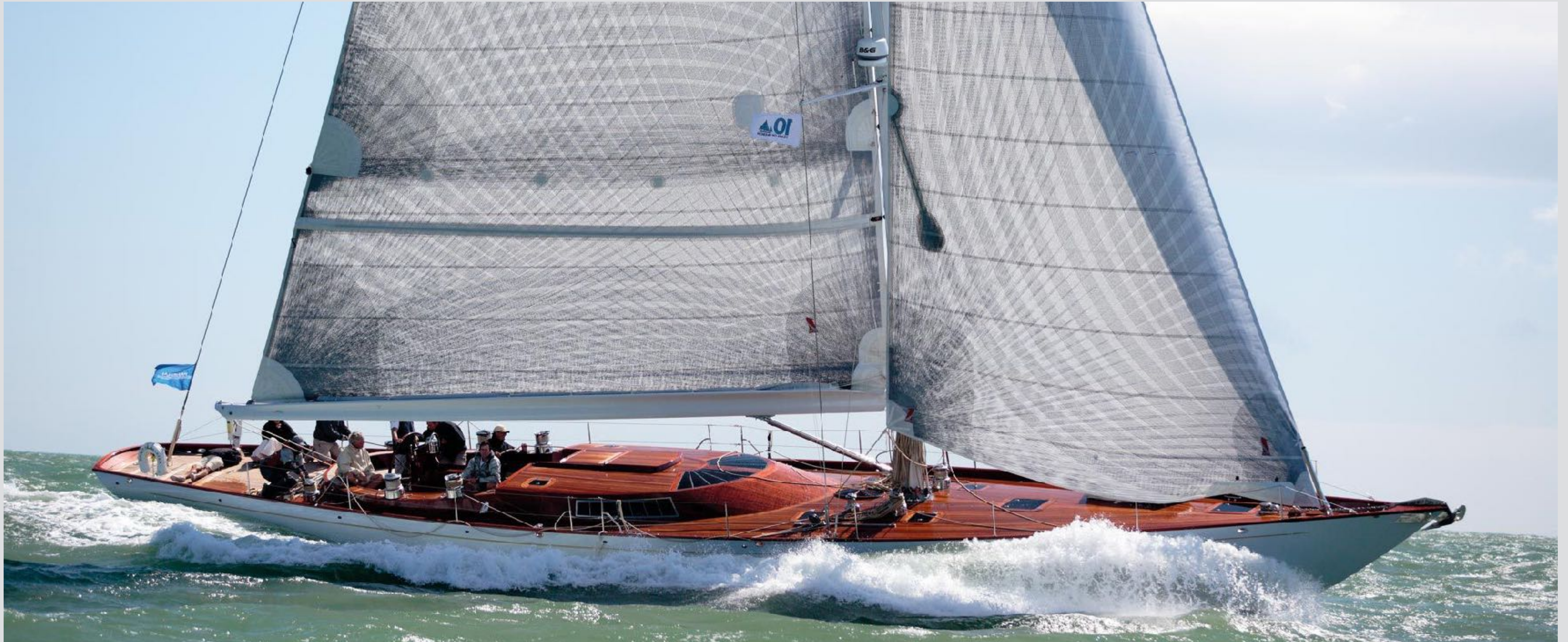
21ST CENTURY SAIL MADE FROM FIBER COMPOSITE MATERIAL (North Sails, 3DL ,URL < http://www.nauticexpo.de , 07.12.2017)
