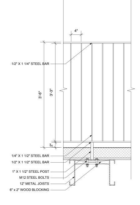
ROOF RAILING DETAIL
