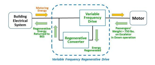
Figure LE-11. Escalator Variable Frequency Regenerative Drive
