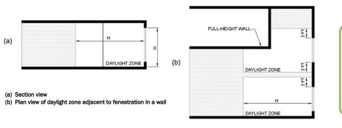
For Daylight Zone under Fenestration located in a Rooftop Monitor following ECC, refer to Figure C405.2.3.2(2) and C405.2.3.2(3).
