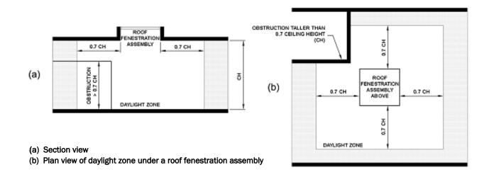
Figure LE-7. Daylight Zone Under a Roof Fenestration Assembly
