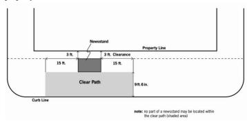
Illustration 4: Typical full block front plan showing clearance from corners and curb of streets.
