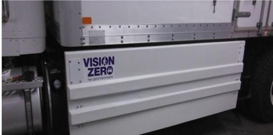
In May 2014 DCAS partnered with the Volpe Center at US DOT to conduct an assessment of truck sideguard technology. Sideguards are rails placed between the front and rear wheels on trucks that can protect bicyclists, pedestrians and motorcyclists in the case of a collision.
