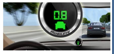
board. Hardware included in the pilot program are the vision sensor unit, a high-quality audio alert buzzer, and an "EyeWatch" display and control kit (pictured). Using image recognition technology, the Mobileye units can warn the driver if their vehicle is at risk of striking a pedestrian, bicyclist, or a vehicle in front or in an adjacent lane.
