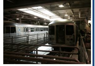
into the school some distance away from the closest tracks through an elaborate towing and crane operation. Students are able to walk into and under the cars to conduct mechanical and electrical lab exercises on them.
