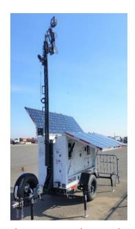
enabling zero emission lighting at night. The units are silent, low maintenance, use improved LED lighting, and can be programmed to turn on and off remotely. The units offer the prospect of zero emissions and vastly reduced maintenance costs. As a contingency, we have procured some units with backup emergency fuel tanks in case of extended emergency operations.
