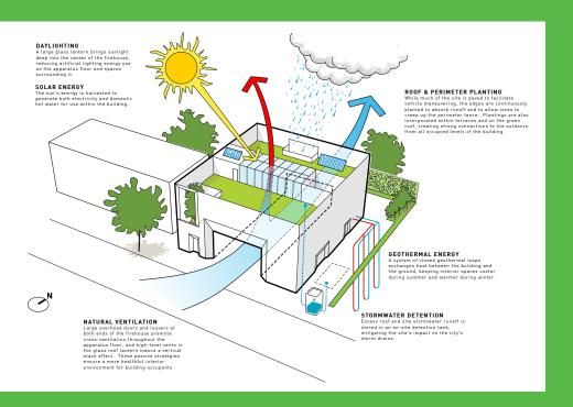
Leverage site and envelope response. Site tactics (the reduction of building heating and cooling loads through orientation and shading) can amplify energy efficient envelope design (highly insulated, with daylight and breeze capture). These tactics, carefully coordinated, can create improved indoor and outdoor environments while reducing energy use and GHG emissions at modest or no cost.
