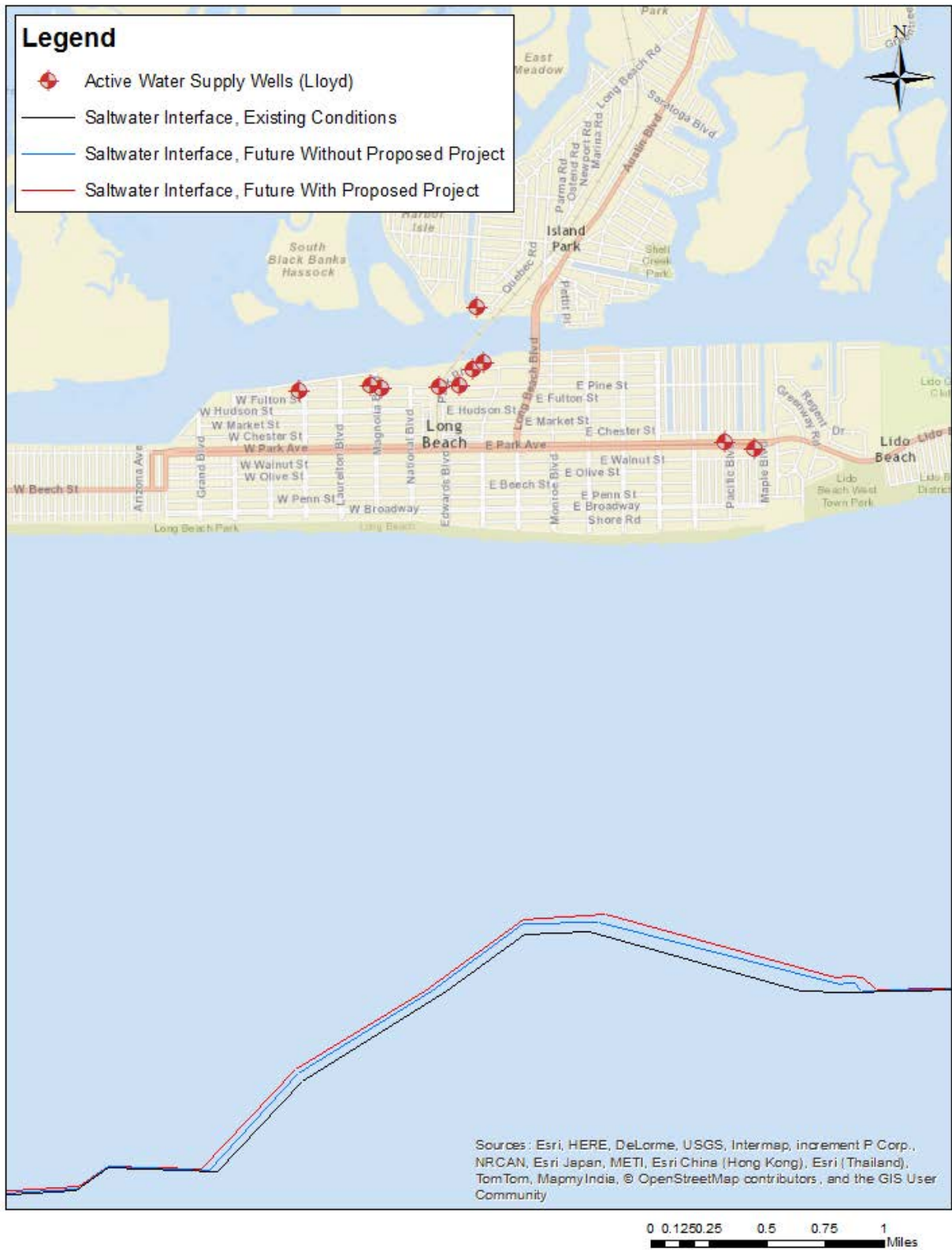
Figure 3.5-38: Saltwater Interface Location, Lloyd Aquifer (South Shore Near Long Beach) - Scenario D (62 mgd for 5 Years)
