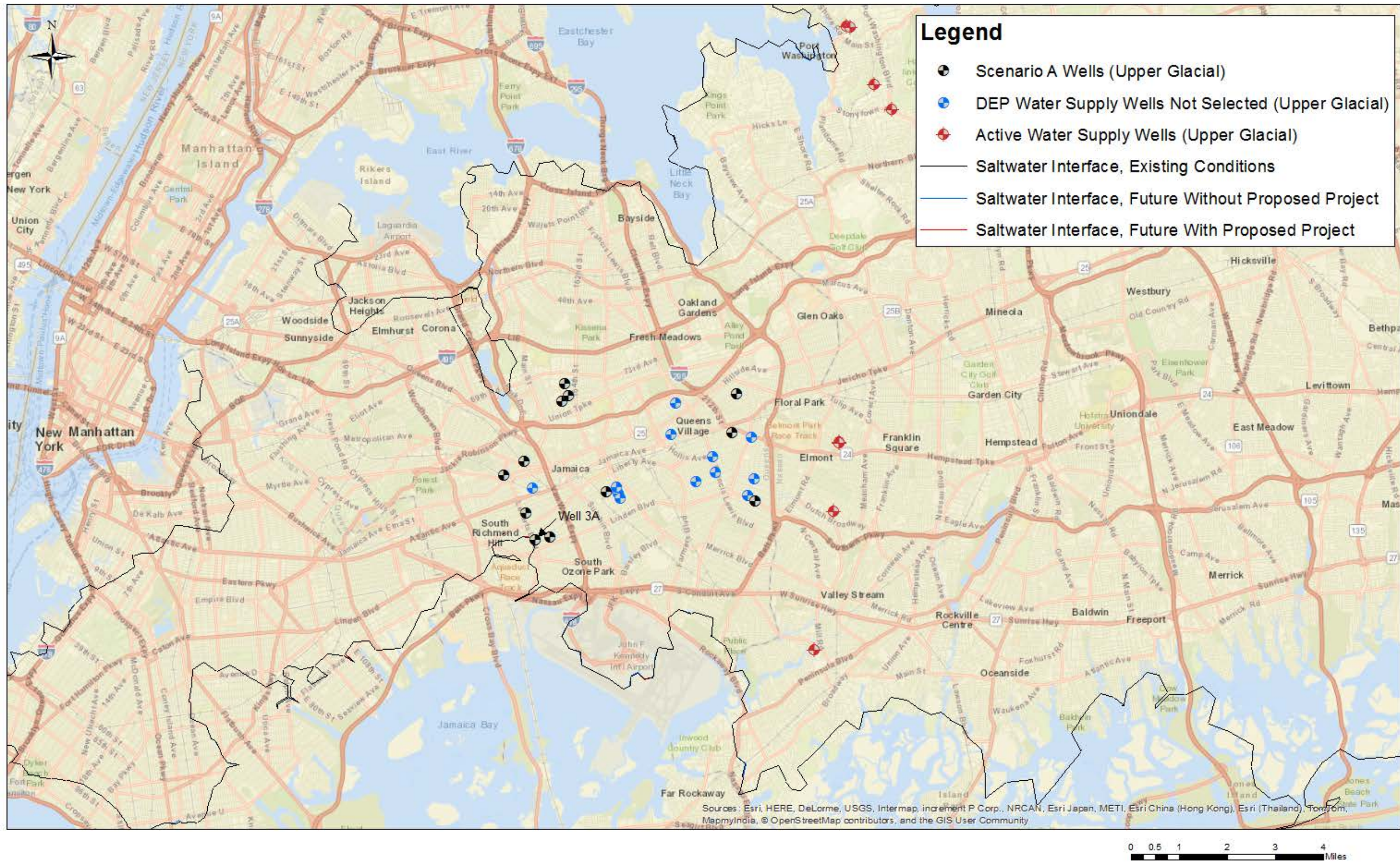
Figure 3.5-15: Saltwater Interface Location, Upper Glacial Aquifer - Scenario A (68 mgd for 1 Year)
