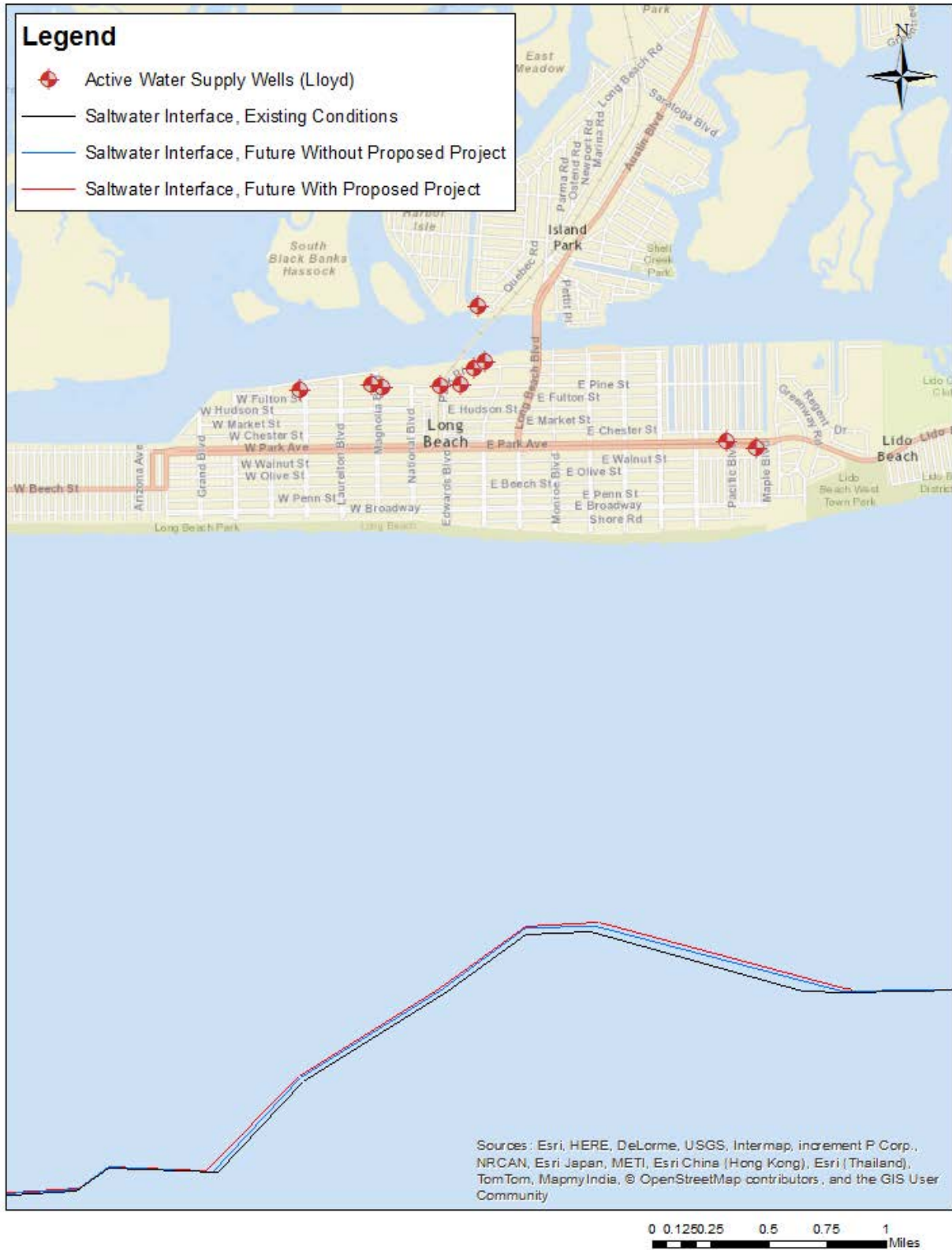
Figure 3.5-37: Saltwater Interface Location, Lloyd Aquifer (South Shore Near Long Beach) - Scenario C (68 mgd for 3 Years)
