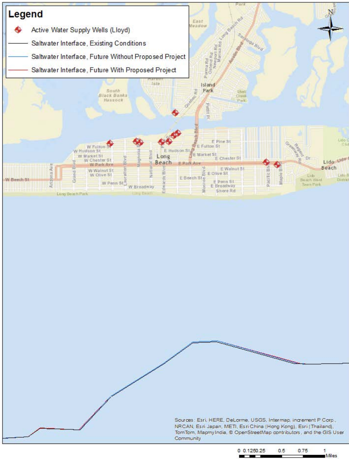
Figure 3.5-35: Saltwater Interface Location, Lloyd Aquifer (South Shore Near Long Beach) - Scenario A (68 mgd for 1 Year)
