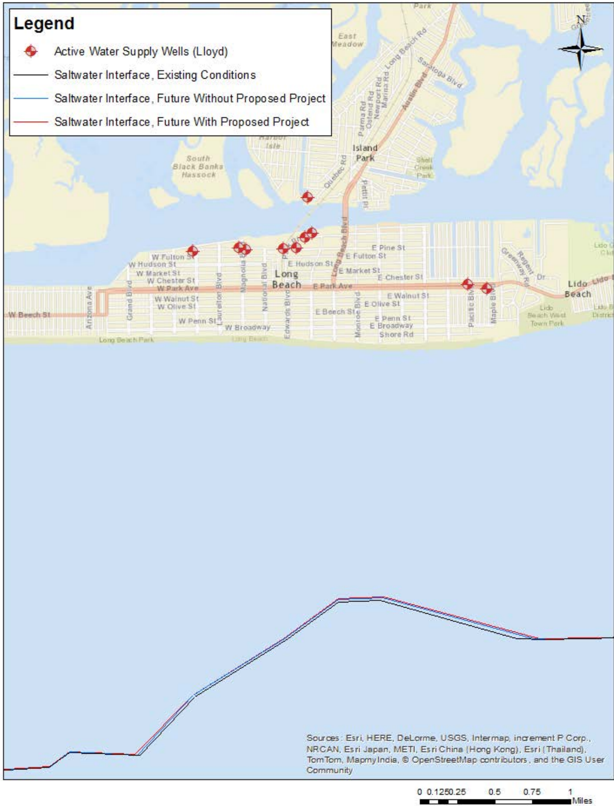
Figure 3.5-36: Saltwater Interface Location, Lloyd Aquifer (South Shore Near Long Beach) - Scenario B (68 mgd for 2 Years)
