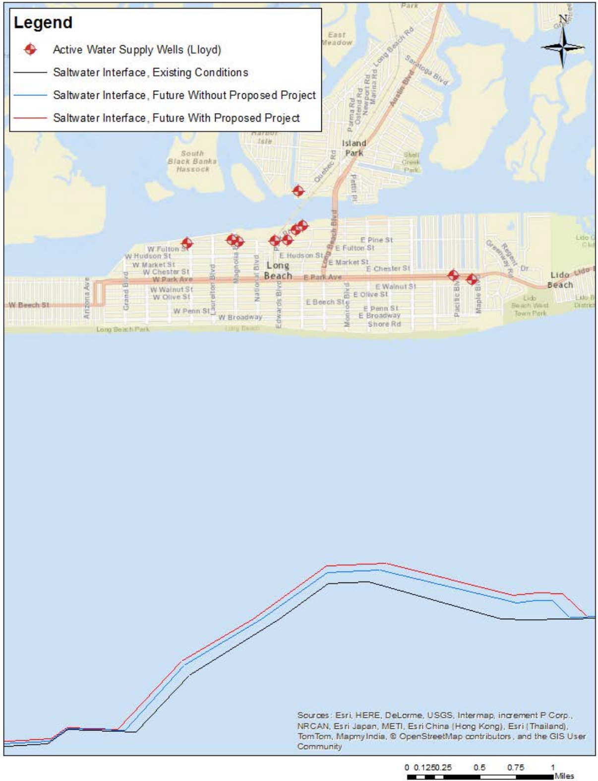
Figure 3.5-39: Saltwater Interface Location, Lloyd Aquifer (South Shore Near Long Beach) - Scenario E (62 mgd for 10 Years)
