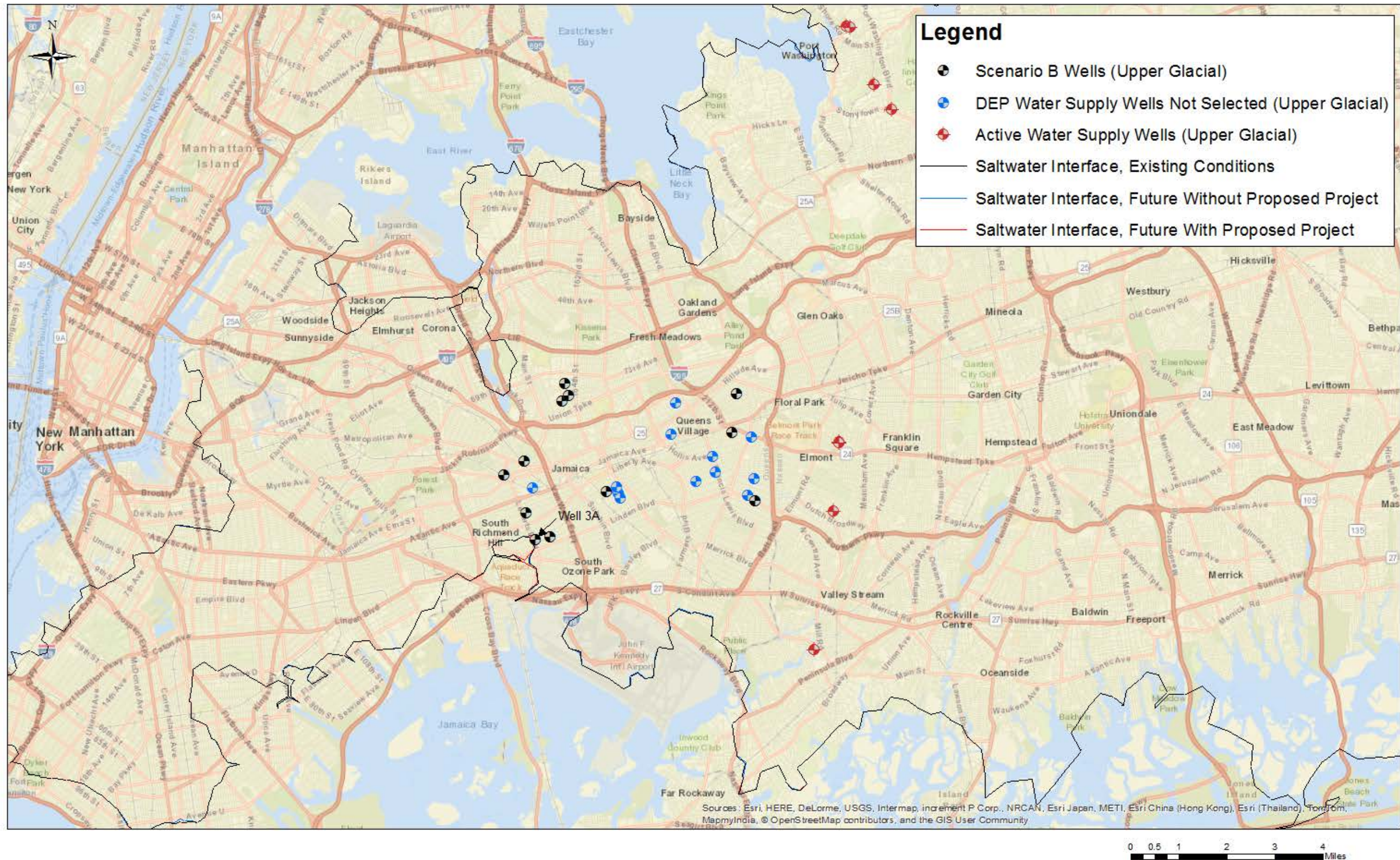
Figure 3.5-16: Saltwater Interface Location, Upper Glacial Aquifer - Scenario B (68 mgd for 2 Years)
