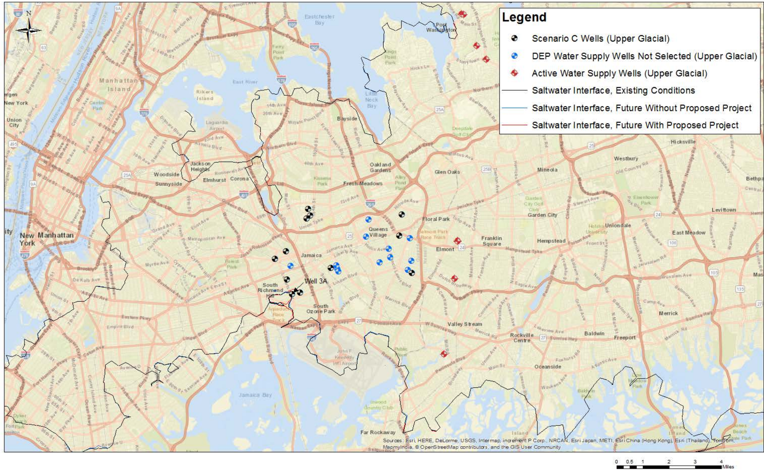
Figure 3.5-17: Saltwater Interface Location, Upper Glacial Aquifer - Scenario C (68 mgd for 3 Years)
