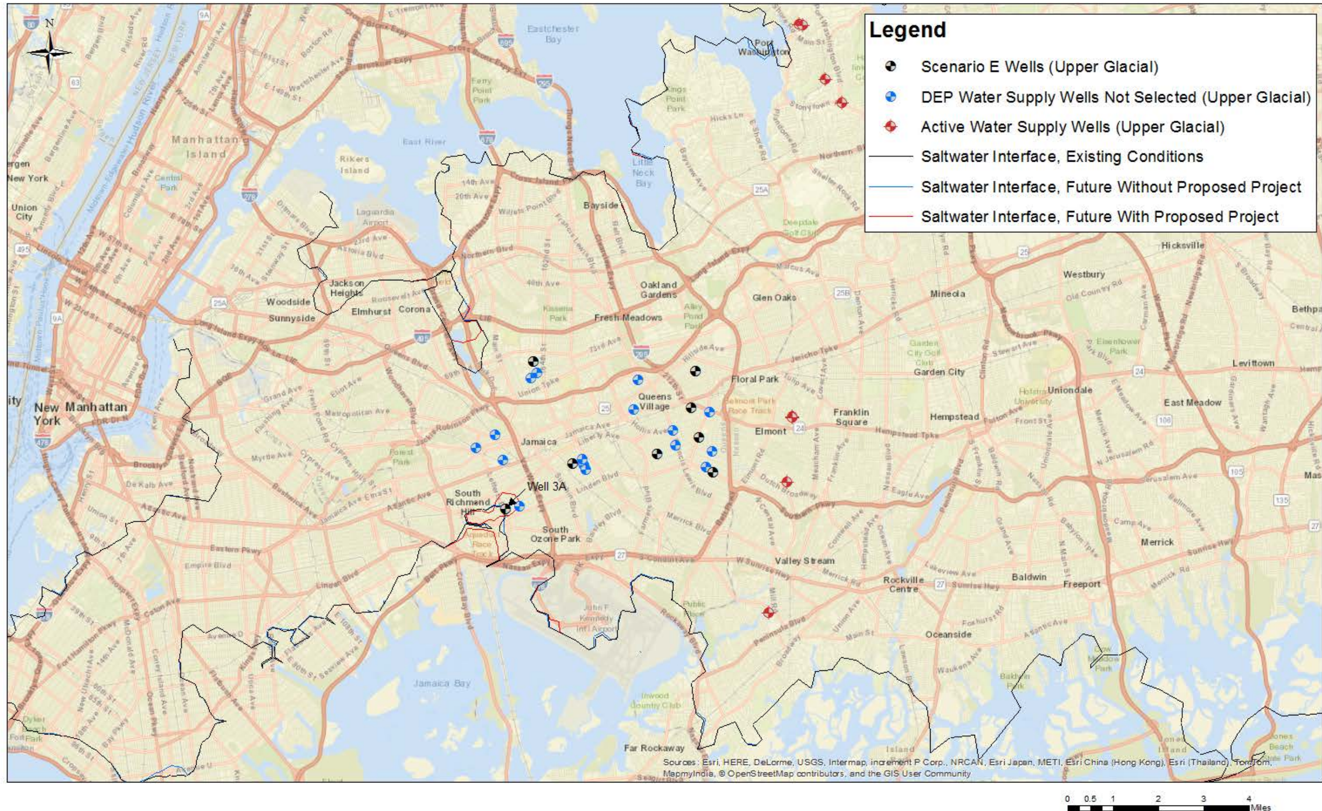
Figure 3.5-19: Saltwater Interface Location, Upper Glacial Aquifer - Scenario E (62 mgd for 10 Years)
