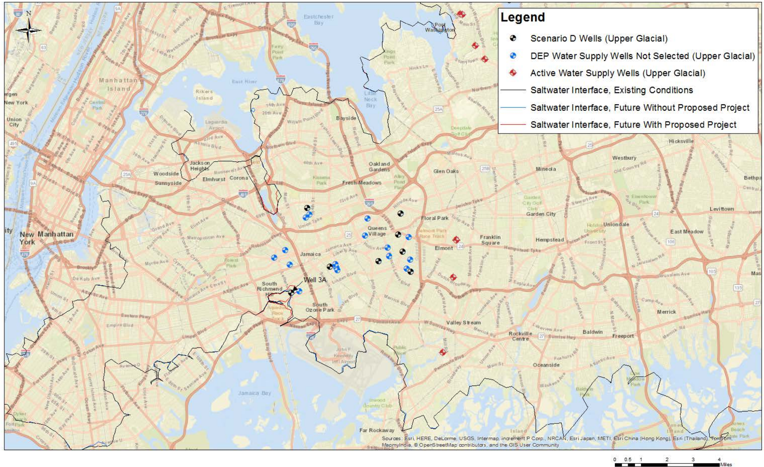
Figure 3.5-18: Saltwater Interface Location, Upper Glacial Aquifer - Scenario D (62 mgd for 5 Years)
