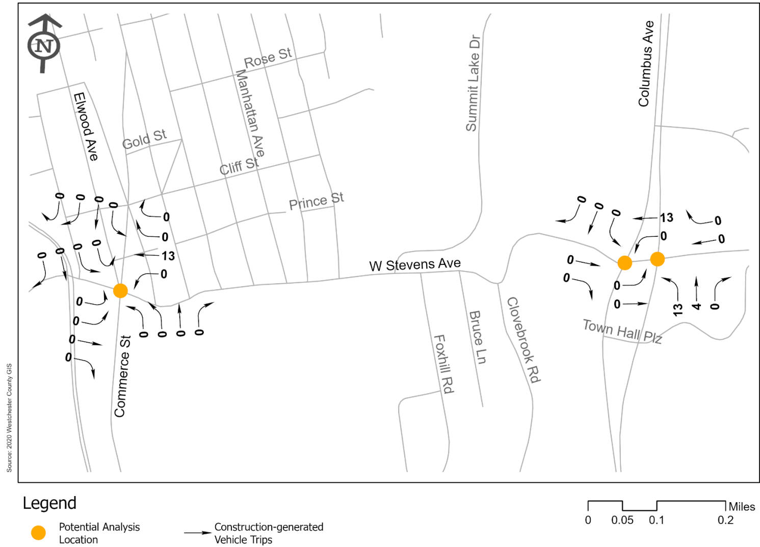
Figure 3.10-34. Inset H – Construction-Generated Vehicle Trips – Fourth Quarter of 2027 PM Construction Traffic Peak Hour
