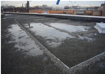
The rooftop was partitioned to examine three types of blue roofs and an uncontrolled reference area.
