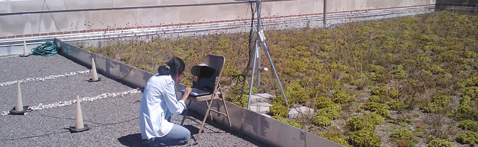
Monitoring of the blue roof (left), green roof (right) and an uncontrolled section (not shown) at PS 118.
