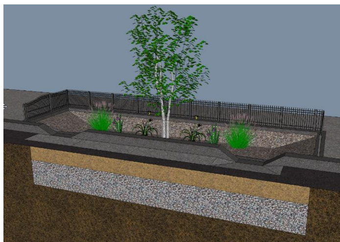
Example design of an enhanced tree pit with open curb cuts.
