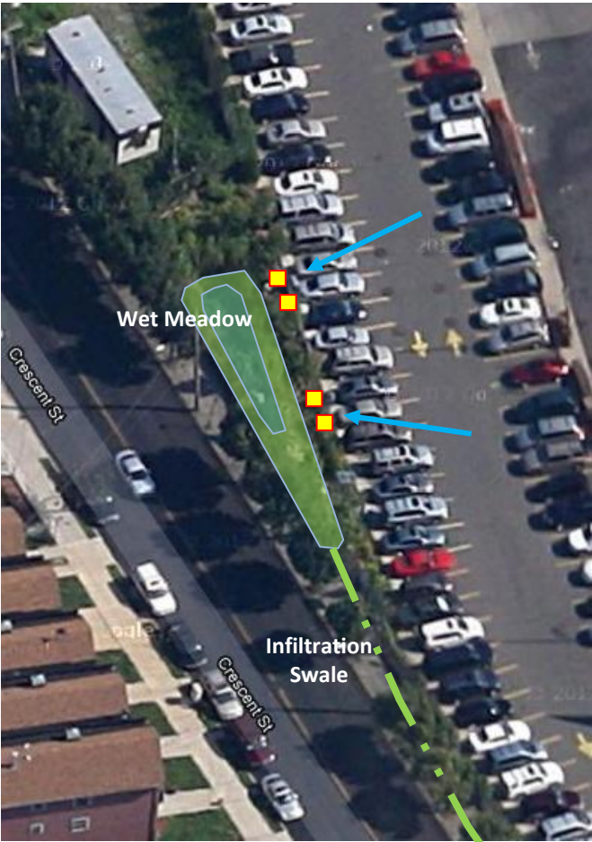
Stormwater runoff from the MTA parking lot is diverted to the wet meadow via perimeter catch basins. Excess water overflows into an infiltrating bioswale.
