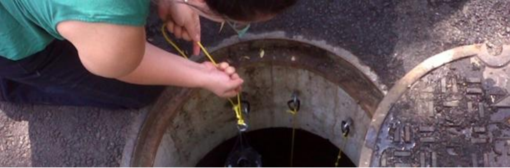
Researcher lowering a water quality sampler into a subsurface system at the Bronx River Houses.
