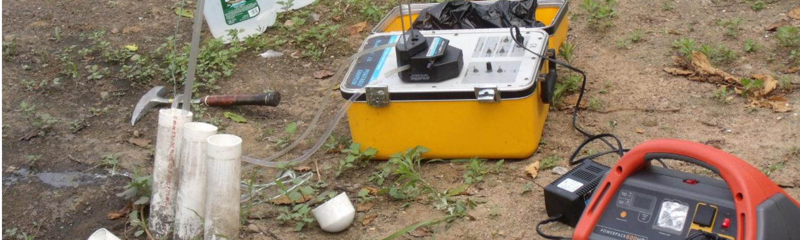
Water quality sampling equipment at a bioretention facility, drawing water from wells that capture runoff after it has infiltrated through the soil.
