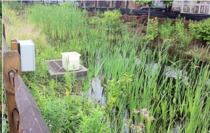
Established vegetation in the wet meadow pilot at the Spring Creek MTA Bus Terminal under saturated conditions. Monitoring equipment was installed at the outlet (shown on right) to measure outflow.
