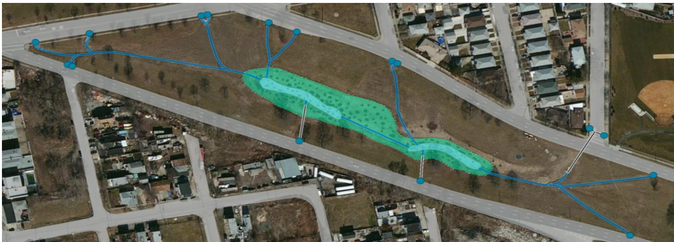
Map illustration of bioretention cells and inflow swales at the North & South Conduit Avenues pilot.
