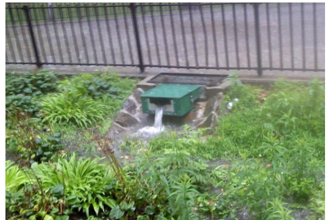
Runoff flows from a curb cut through a weir box where flow is measured as it enters a bioretention pilot.
