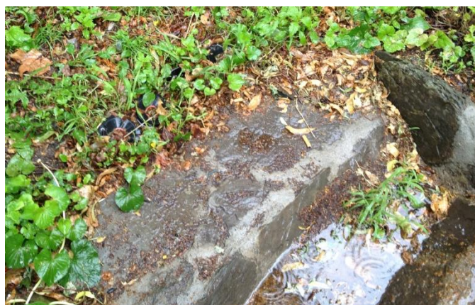
Subsurface sampling canisters, partially shrouded by vegetation, capture water flowing into a bioretention area, then seal once they are full.
