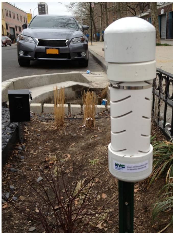
The time lapse camera (back-left) in this greenstreet is recording changes in vegetation over the course of the year as well as the presence of birds or valuable insects. The temperature sensor (foreground) is being used to compare air temperatures above the greenstreet surface to temperatures along a nearby standard sidewalk.
