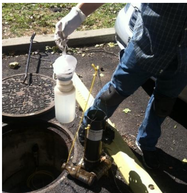
A water quality sampling canister being assembled before installation in an outlet manhole at Bronx River Houses.
