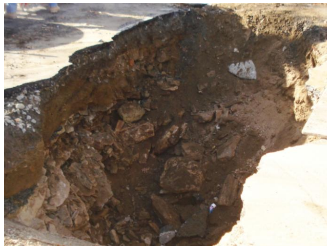
Smaller and fractured rock was more common under the north parking lot system, along with less clay and more loamy soil.
