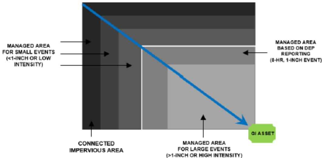
**Schematic of Connected v. Managed Impervious Area for GI Assets**
