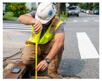
Measuring debris in catch basin for Loading Rate Study
