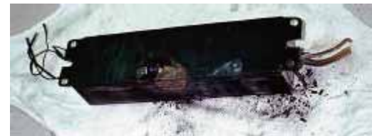
This ballast sparked a fire at a Southern California school in 1999.
