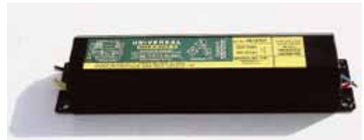
An intact ballast from a typical pre-1979 fluorescent light fixture.
