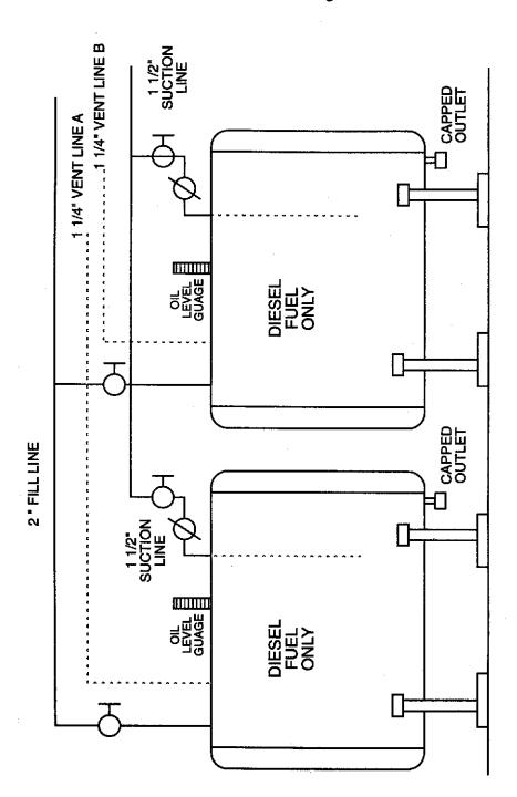
(1) Schematic drawing for two (2) 275 gallon tanks.
