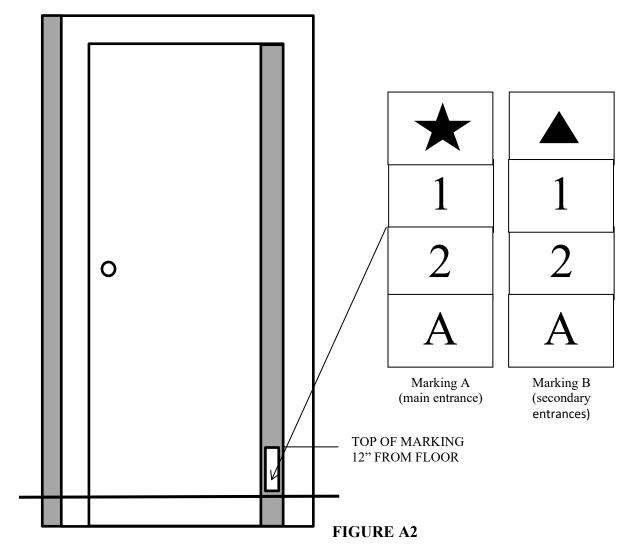
Figure A2 depicts the location, vertical configuration and star and triangle symbol of the fire emergency marking for a dwelling unit designated as 12A having more than one entrance door. Each entrance door is required to be marked separately.
