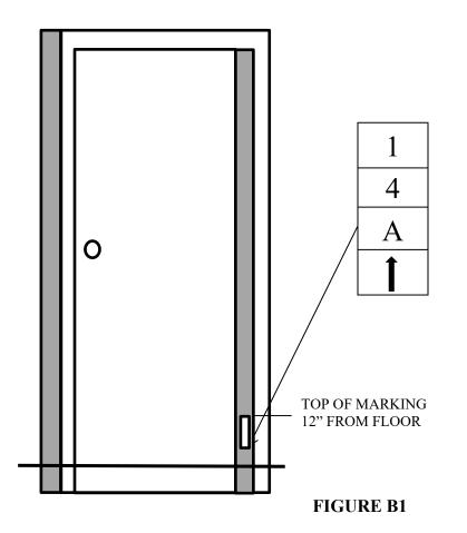
Figure B1 depicts the location, vertical configuration, arrow symbol and arrow directions for a two-floor *multi-floor dwelling unit* designated 14A, having a single entrance door. The upward-pointing arrow indicates that the dwelling unit is a *multi-floor dwelling unit* having living space on the entry floor and on the floor above this floor.
