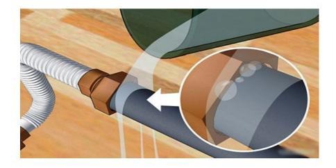
A lighted flame (for example, a match or a propane torch) MUST NEVER be used when checking a connection for a natural gas leak.
