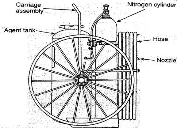
**Fig.3. Wheeled-type cylinder-operated dry chemical PFE**
