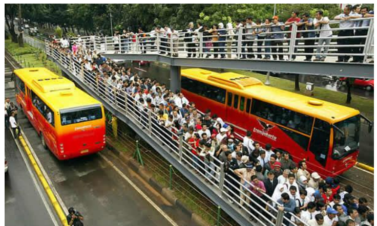
BRT System with physically separated bus-only lanes and boarding platform
