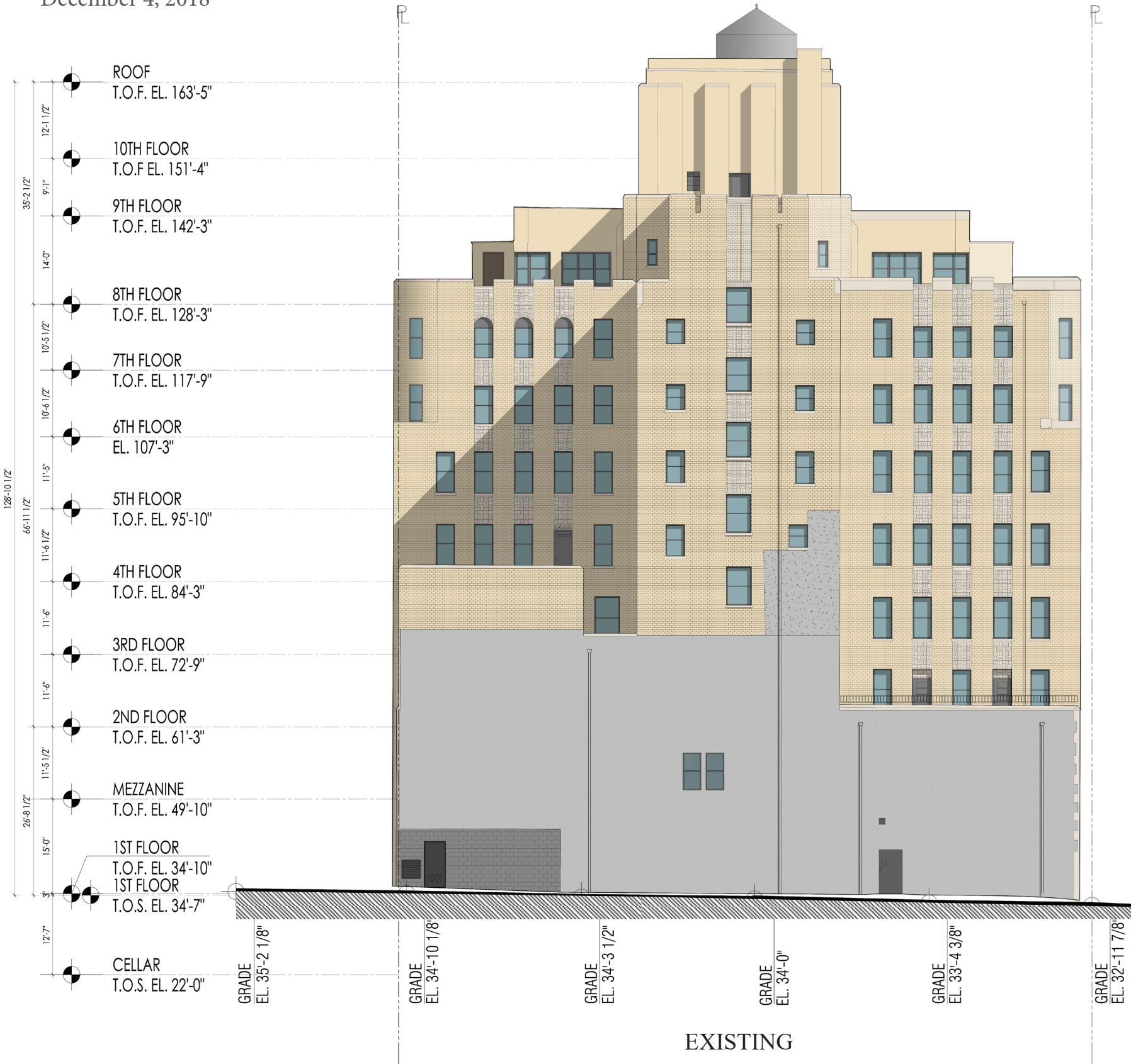
2 WEST BUILDING ELEVATION (Lot 45) SCALE: 3/32" = 1'-0" 0 5' 10' 20'
