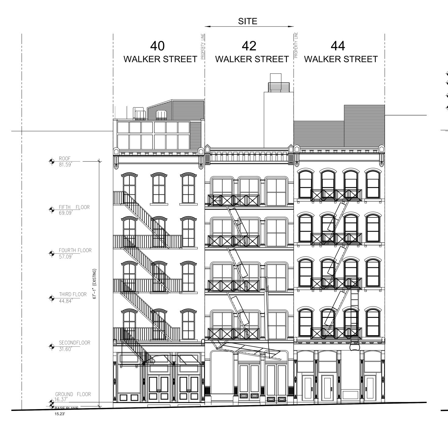
SITE 40 44 WALKER STREET WALKER STREET WALKER STREET MECHANICS ELEVATOR BULKHEAD ROOF 84'-9"AS PER LPC DOCKET #16-4406 / CNE #16-7761 42" GLASS -RAILING -NEW SIXTH FLOOR ROOF (UNDERSIDE OD STRUCTURE) 90.25' FIFTH FLOOR ROOF 81.59' FOURTH FLOOR 57.09' THIRD FLOOR
