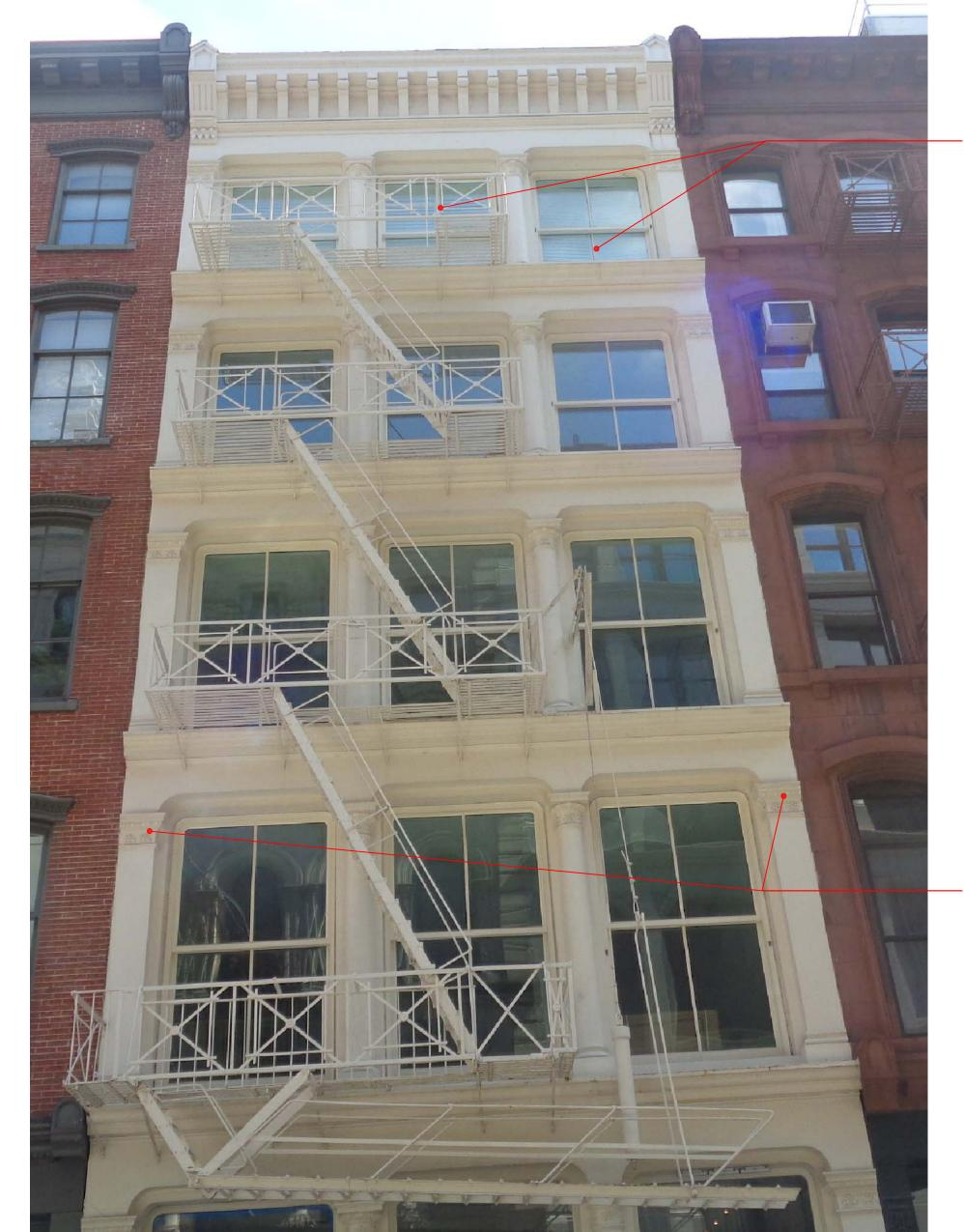
TWELVE EXISTING WINDOWS AT SECOND THROUGH FIFTH FLOOR ARE REPLACED WITH TWELVE TWO-OVER-TWO DOUBLE HUNG WOOD WINDOWS WITH CURVED CORNERS AT THE TOP OF THE SASHES AT EXISTING OPENINGS.
