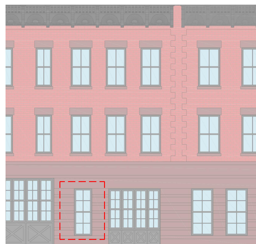
DOUBLE HUNG WINDOWS AT EXISTING BUILDING
