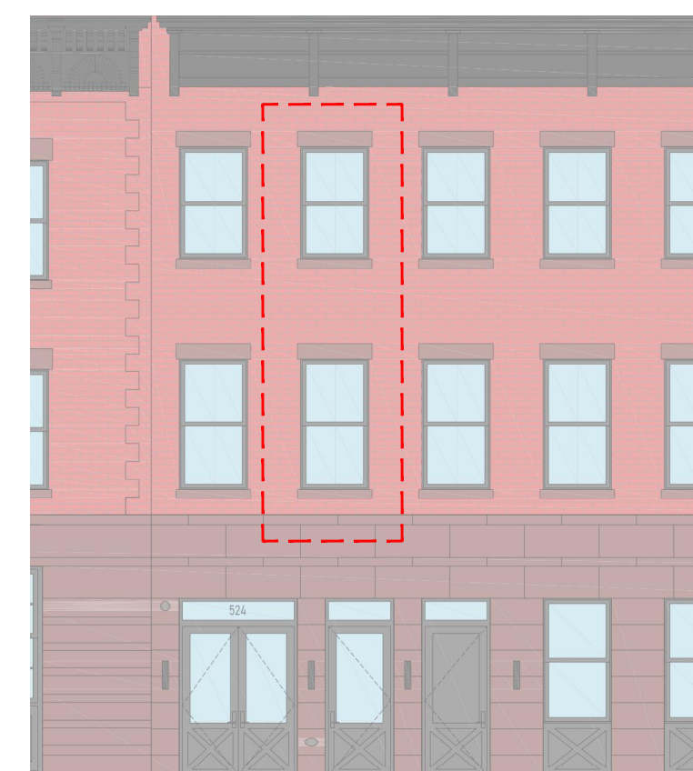
DOUBLE HUNG WINDOWS AT NEW BUILDING
