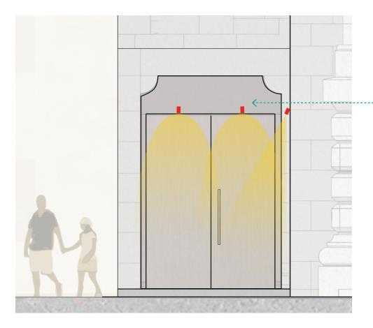
small adjustable fixtures to be mounted on vertical surface to floodlight garage area without creating scallops on the
