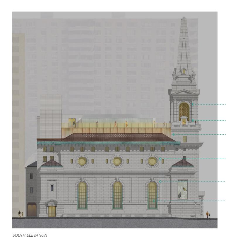
glow from interior to highlight lantern behind reconstructed lattice
