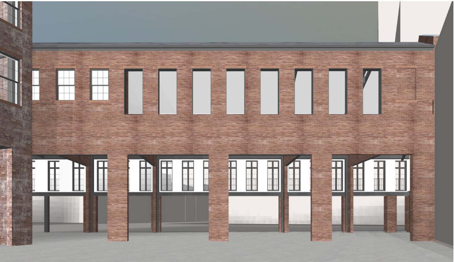
CURRENTLY PROPOSED 9TH AVE BLDG REAR WALL - EXISTING REAR WALL TO REMAIN AND BE RESTORED.
