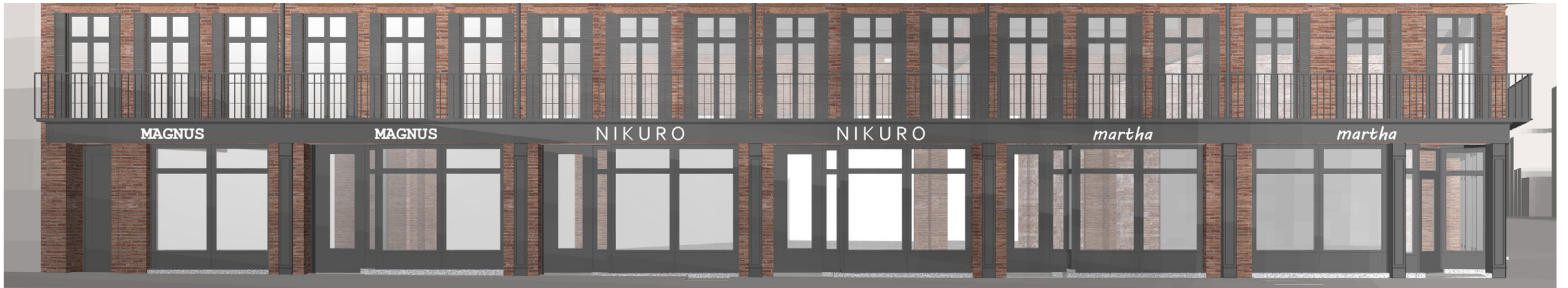
CURRENTLY PROPOSED -HISTORICAL SIGNAGE BAND WITH NEW BALCONETTE ABOVE. BRICK PIERS EXTEND TO GROUND AT PARTY WALL LOCATIONS.
