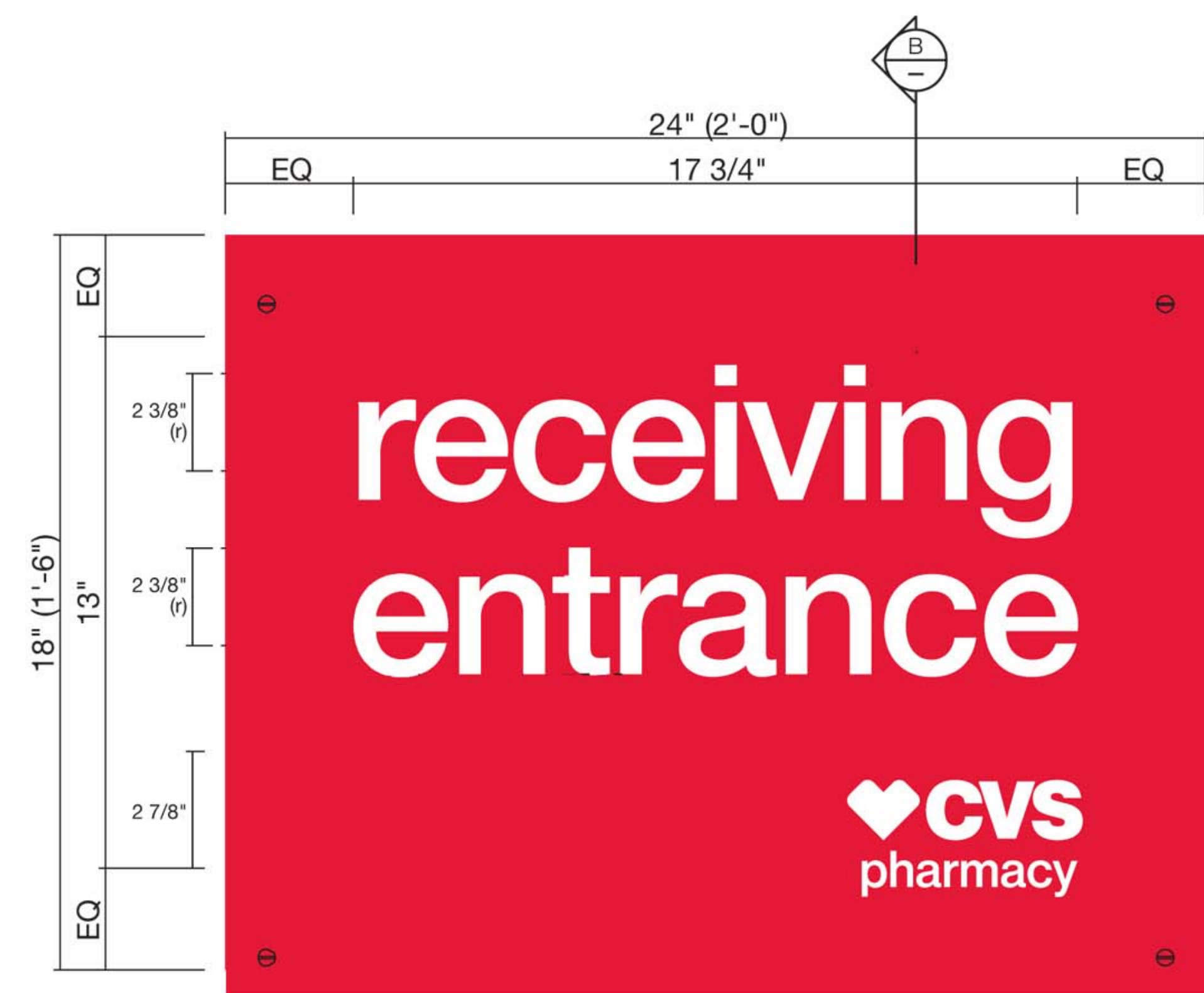
A Sign Elevation - Front View Scale: 2"=1'-0"
