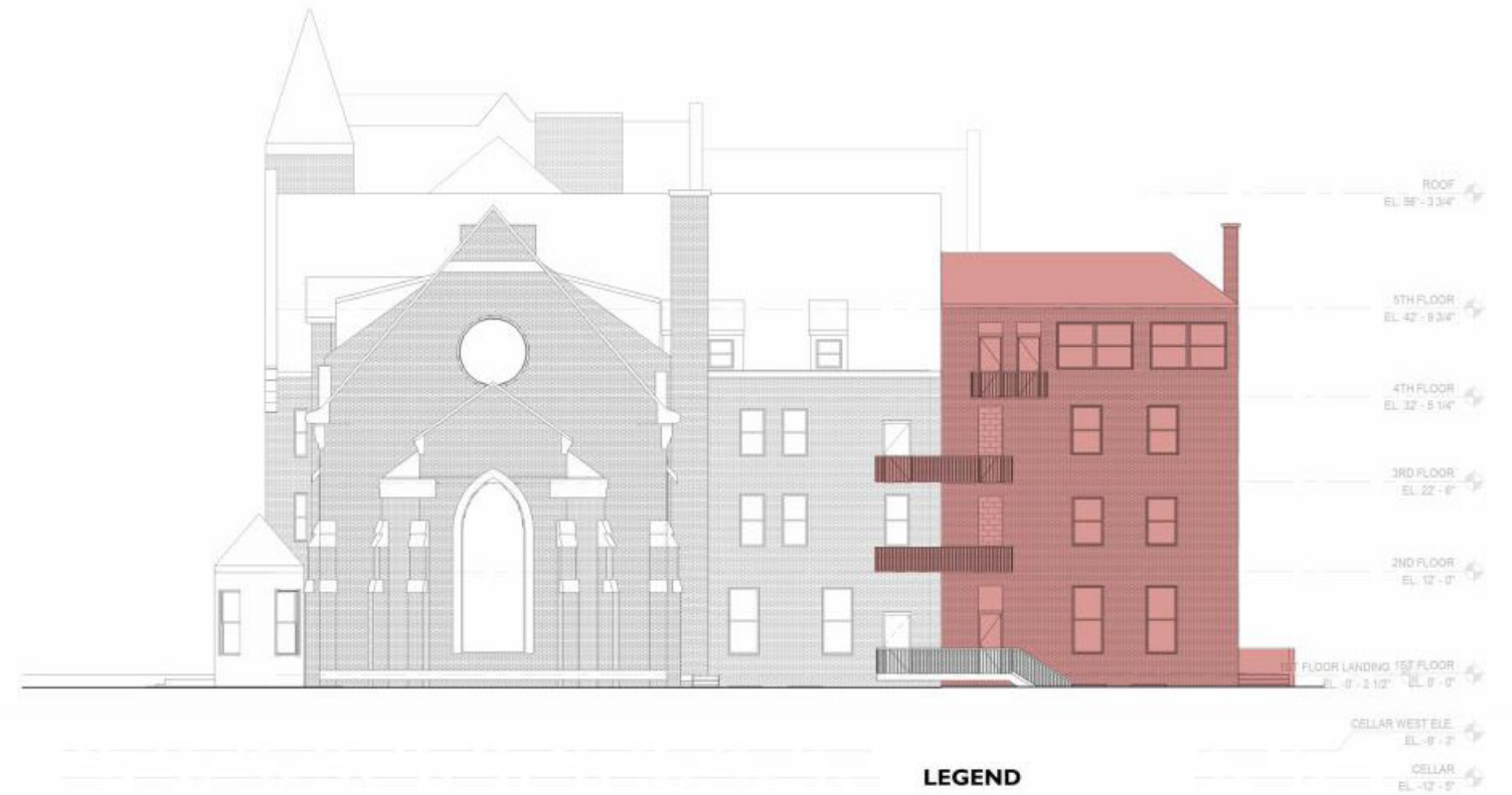
WEST ELEVATION REMOVAL
