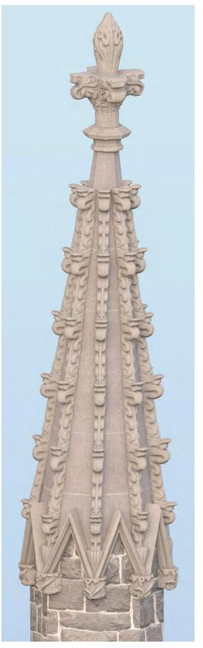
Axonometric View - Proposed Tower #1 and Tower #4. Renders of Proposed GFRP Replacement. PROPOSED FINIAL REPAIRS
