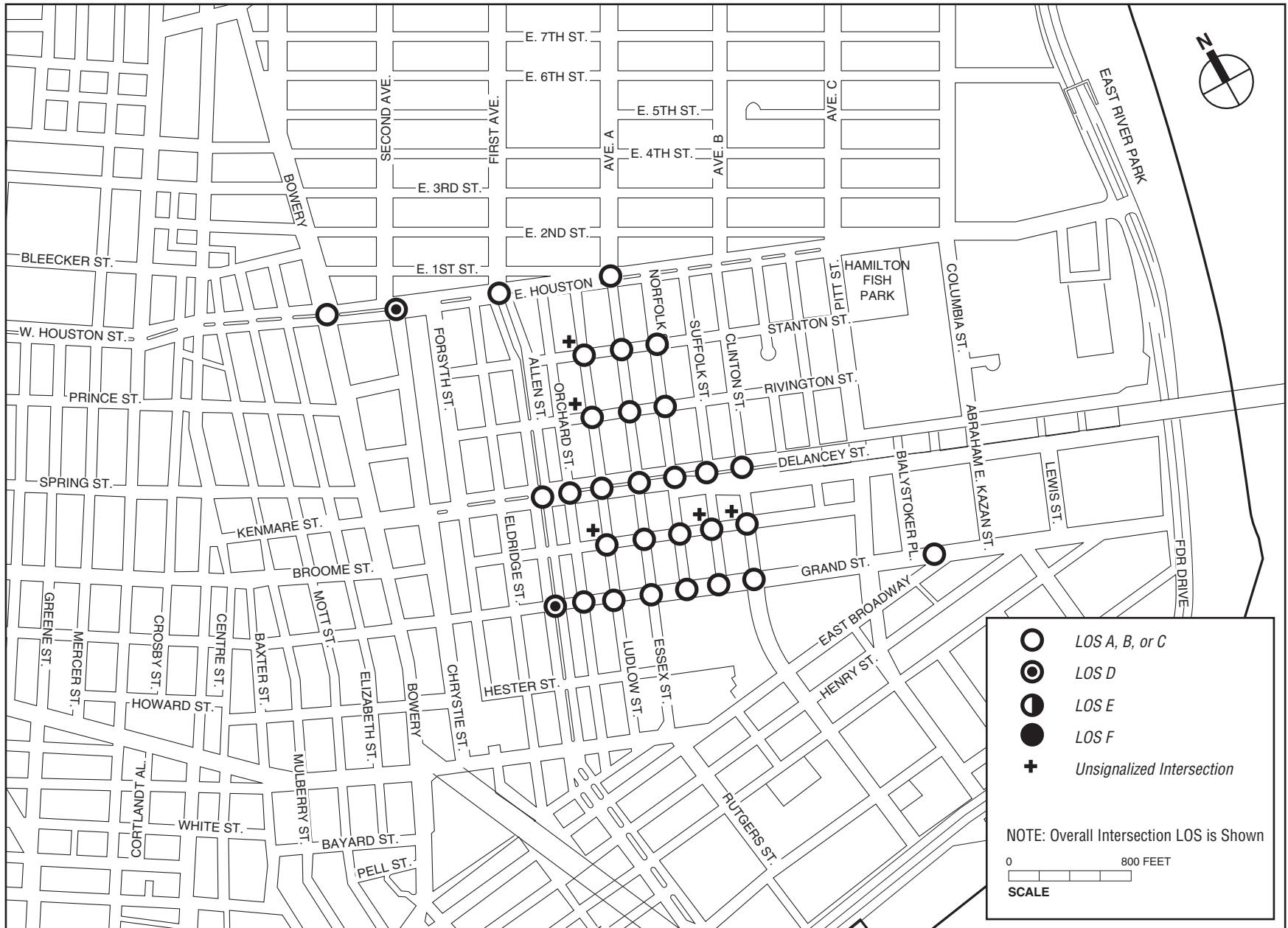
Existing Traffic Levels of Service - Overall Intersections Weekday Midday Peak Hour Figure 13-5a
