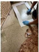
Technician using template to take dust wipe sample. Sample packaged in rigid centrifuge tube. (Building 7 – 131 Ten Eyck Walk. Apt 2C)
