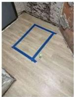
Painters tape used a template to take dust wipe sample. Sample packaged in hard shell container. (Building 2 – 210M W 153rd St., Library)
