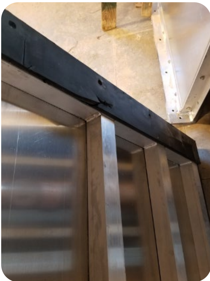
Coney Island 4/5: Example of gasket damage that has to be avoided
