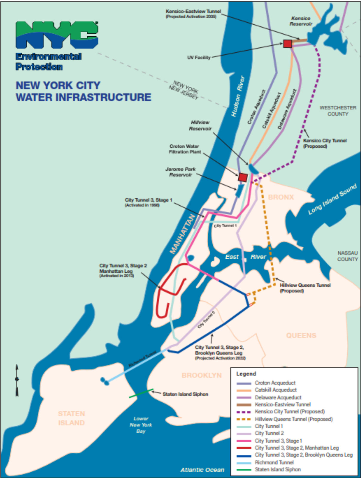
Figure 5-2: New York City Water Conveyance Infrastructure
