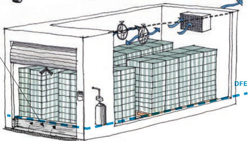
Move ethylene gas supply above the DFE
