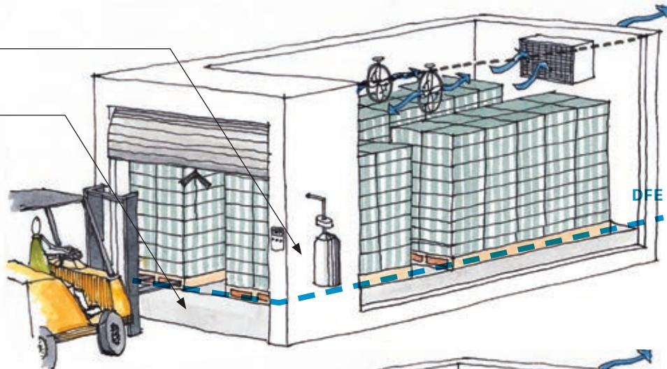
Install deployable flood gates at opening of each ripening room and seal exterior walls so that they are impermeable to water.
