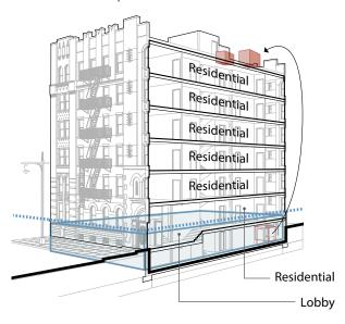
No or partial reduction in NFIP premiums. Residential use and partial critical systems remain located below the DFE and the structure is not filled to the lowest adjacent grade. Dry floodproofing is not permitted at residential use. Lowest occupiable floor is below the DFE.
