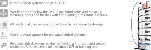
Dry floodproof partial basement level at mechanical room.
