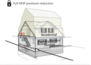
No or partial reduction in NFIP premiums. Residential use and critical systems remain located below the DFE and the structure is not filled to lowest adjacent grade. Lowest occupiable floor is below the DFE.
