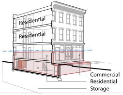
No or partial reduction in NFIP premiums. Residential use remains located below the DFE and the structure is not filled to the lowest adjacent grade. Lowest occupiable floor is below the DFE.
