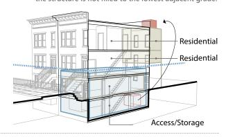
No or partial reduction in NFIP premiums. Residential use remains located below the DFE and the structure is not filled to the lowest adjacent grade. Lowest occupiable floor is below the DFE.
