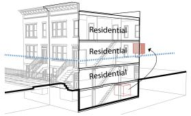
No or partial reduction in NFIP premiums. Critical systems and residential use remain located below the DFE and the structure is not filled to the lowest adjacent grade. Dry floodproofing is not permitted at residential use. Lowest occupiable floor is below the DFE.
