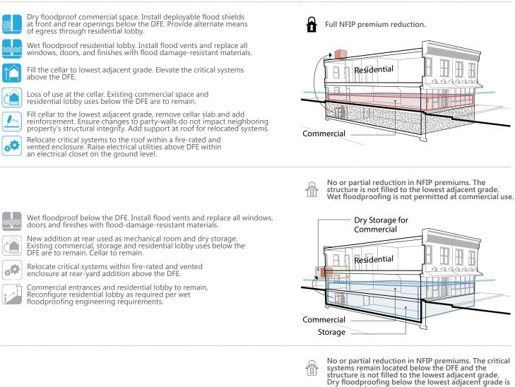
Dry floodproof below the DFE by strengthening the foundation, floors and walls and sealing all penetrations. Install deployable flood shields, front and rear windows, and doors.
