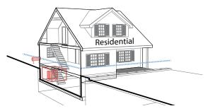
If the DFE is within a few feet of the lowest occupiable floor consider keeping the strucure in place and using flood damageresistant materials below the DFE.
