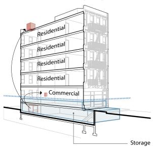
Wet floodproof below the DFE. Install flood vents and replace all windows, doors and finishes with flood damage-resistant materials.
