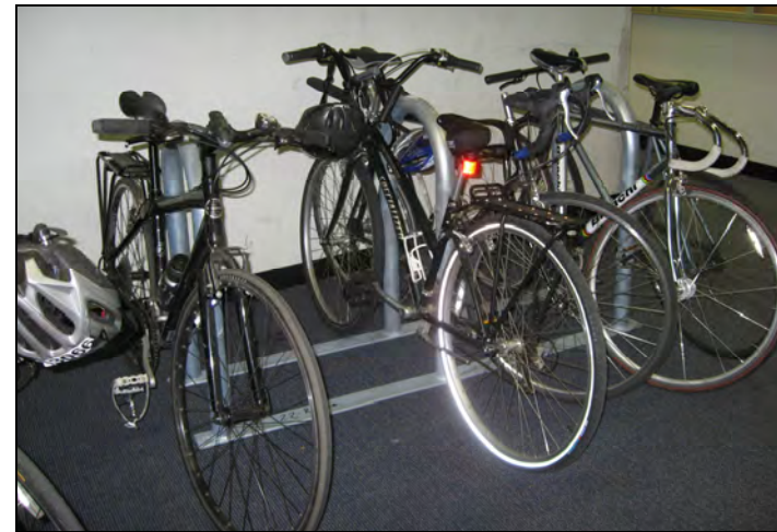
A Multiple “U” rack provided by DCAS for New York City employee use
