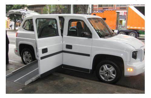
IMAGE 11. MV-1 with ramp shown with ramp extended for wheelchair access. NYC DCP.
