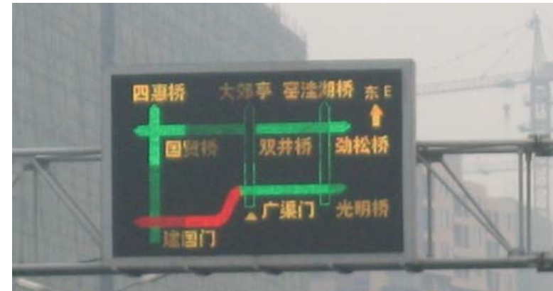
Color-coded real-time traffic congestion message board in Beijing, China. NYC Dept. City Planning
