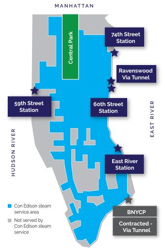
This figure shows the Con Edison steam system service territory. The blue stars indicate the locations of central steam generation plants that are owned and operated by Con Edison. The gray star indicates the cogeneration plant in Brooklyn that is not owned and operated by Con Edison but delivers steam to their steam system in Manhattan according to a contract between both parties.
