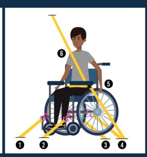
For manual chairs, secure straps on the frame of the chair. Do not secure straps on the wheels.
