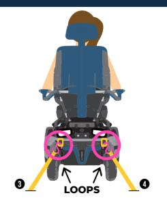
For motorized chairs, secure straps on **loops** at the base of the chair.
