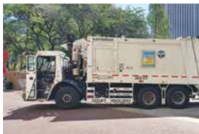
DSNY collector truck with Vision Zero-branded side guard
