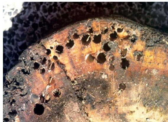
Teredo Damage (holes up to 1/4" diameter)
