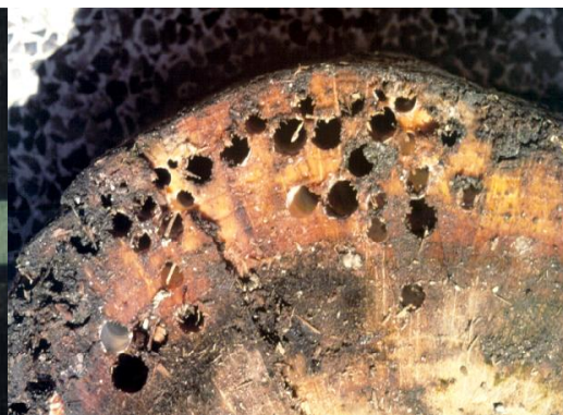
Teredo Damage (holes up to 1/4" diameter)
