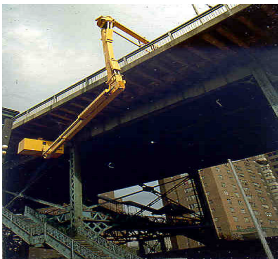
Bridge Inspectors in Snoopers under the Macombs Dam Bridge and the Mill Basin Bridge
