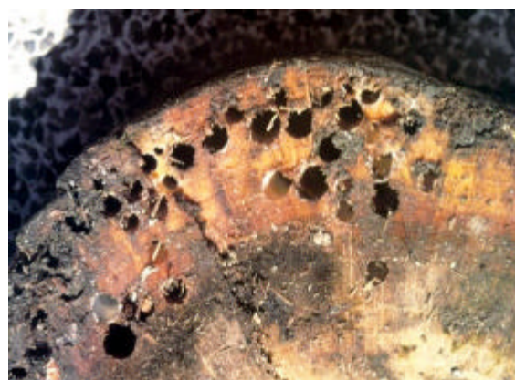
Teredo Damage (holes up to 1/4" diameter)
