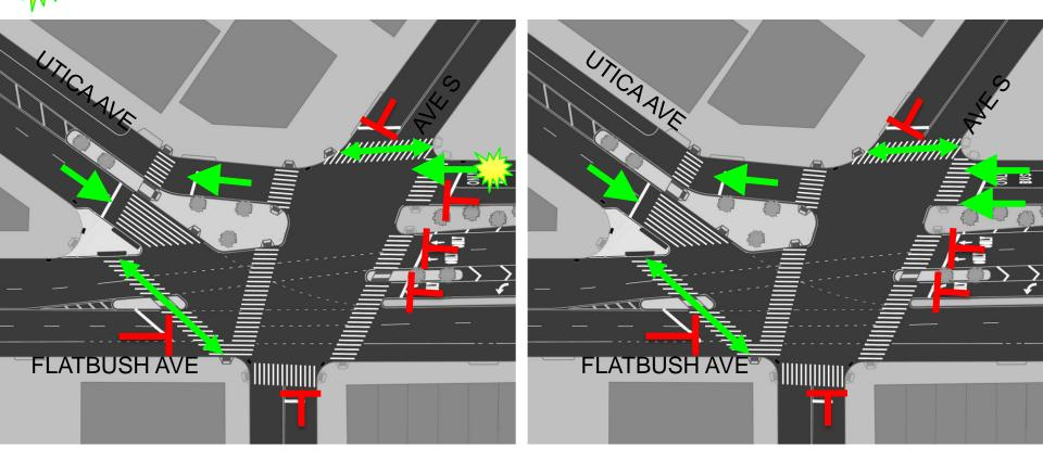
Dedicated Bus Lane Allows for Bus Queue Jump Signal, Giving Bus a 7 Second Head Start onto Single Lane Northbound Utica Ave Before General Vehicle Traffic
