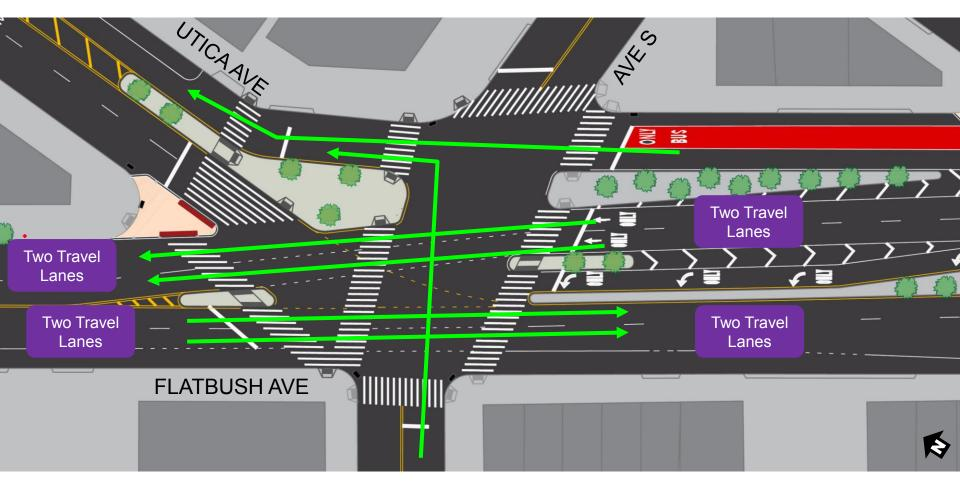
New Concrete and Street Markings Clarify Correct Vehicular Movements
