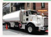
**Crossover mirrors** are a simple way of eliminating a truck driver's front blind spot. They are required by NYS law for trucks, tractors, and tractortrailer or semitrailer combinations, operating with a maximum gross vehicle weight of 26,000 lbs or more, and a conventional cab configuration.
